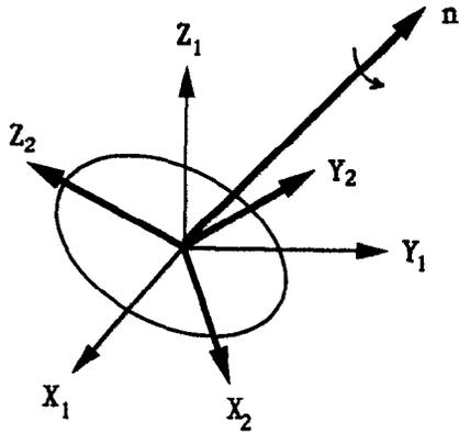
FIG. 1. Illustration of rotation for a real quaternion.
